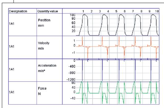
All status variables are dynamically (continually) calculated. In this way, pressure build-up, acceleration and inertia can be precisely simulated. This becomes very interesting if you experiment with cylinder configuration and change one or another variable, for example:
