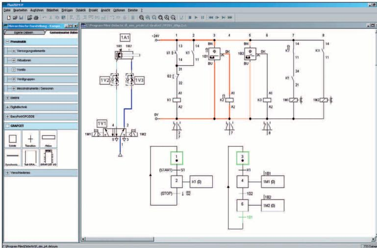
Be confident and well prepared thanks to a dynamic explanation of the new standard. GRAFCET is the new graphic specification language which describes the logical performance and sequence of a control system or a process – regardless of technical conversion in terms of software or hardware.
