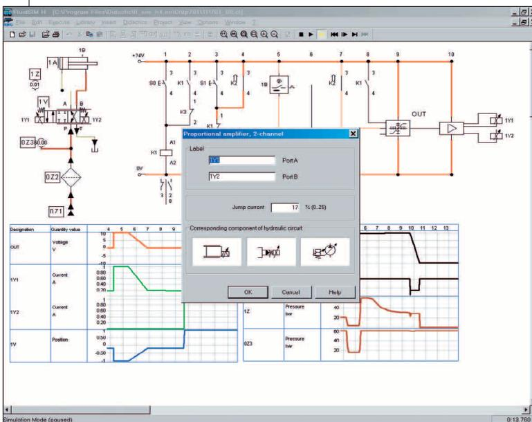
The characteristics of a regulated drive unit under differing, constantly changing loads are complicated. But, together with the dynamic status diagrams, these control circuits and the variables that control them can be very clearly shown with FluidSIM®. A good example is the principle of position control hydraulics.
